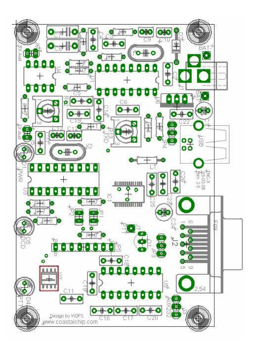
JP1 and JP2 determine the serial port speed for the link between the TNC and the computer. The following settings are allowed:
